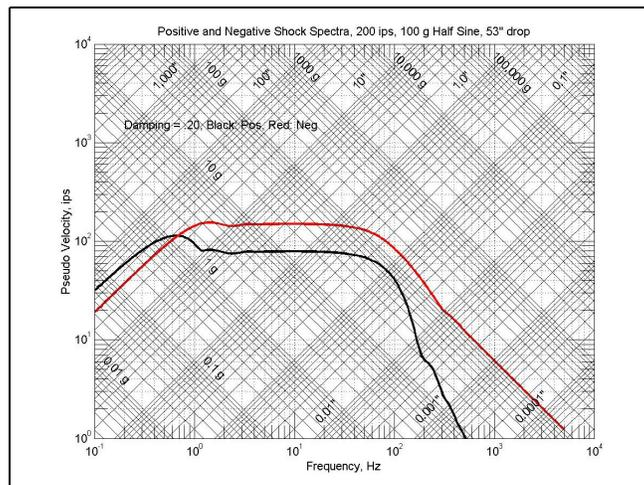
Figure 5b. Positive and negative PVSS for a 20% damped 200 ips, 100 g, half sine. The negative spectrum strongly exceeds (twice) the positive in the high PV plateau.
