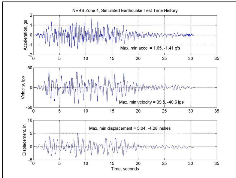
Figure 17a. NEBS Zone 4 Synthesized Earthquake Shock [26]
