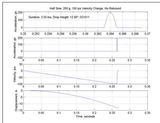
Figure 14a. A 200g, 100 ips half sine shock preceded by a 12.95-inch drop and its integrals.
