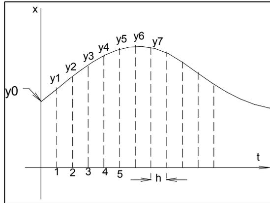
Figure 9. Function of time or acceleration time curve to integrate to velocity.
