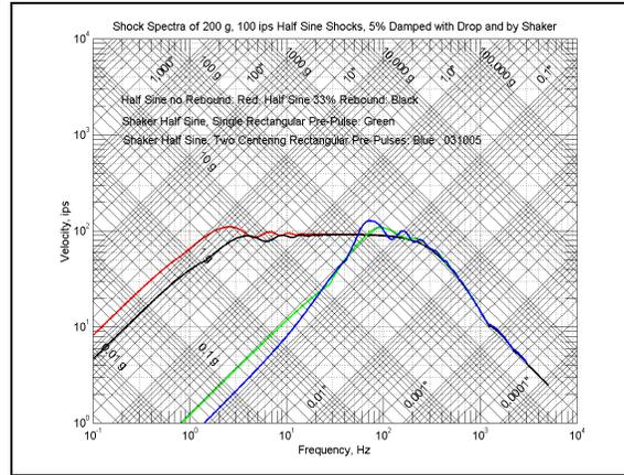
Figure 16b. Shock spectrum comparison of shaker and drop table 200g, 100 ips, half sine shocks for the 5% damped case.
