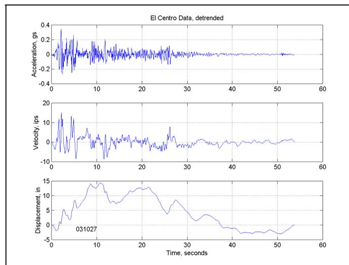
Figure 10c. The El Centro earthquake acceleration detrended and its integrals. Now notice that final displacement is zero, and that peak displacement is a little under 15
