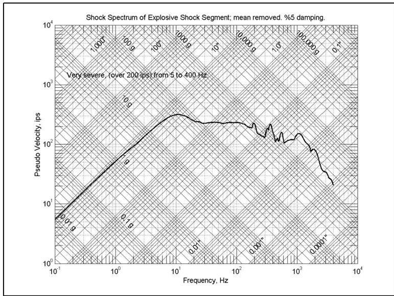
Figure 7a. Five percent damped PVSS of an explosive shock motion.
