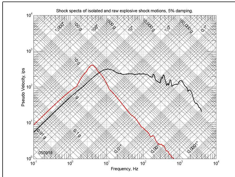
Figure 8b. This shows the PVSS of the Figure 7b motion, and the PVSS of the Figure 8a motion. The isolation is successful.
