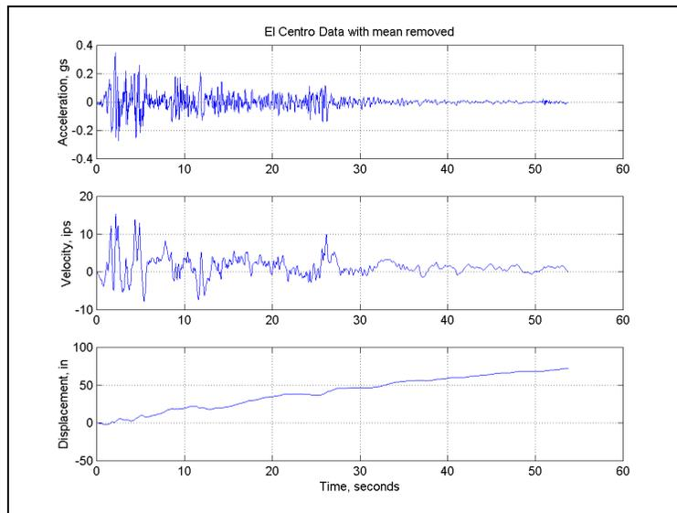
Figure 10b. El Centro with the acceleration mean removed. Note that the velocity ends at zero and now the peak displacement is about 70 inches.
