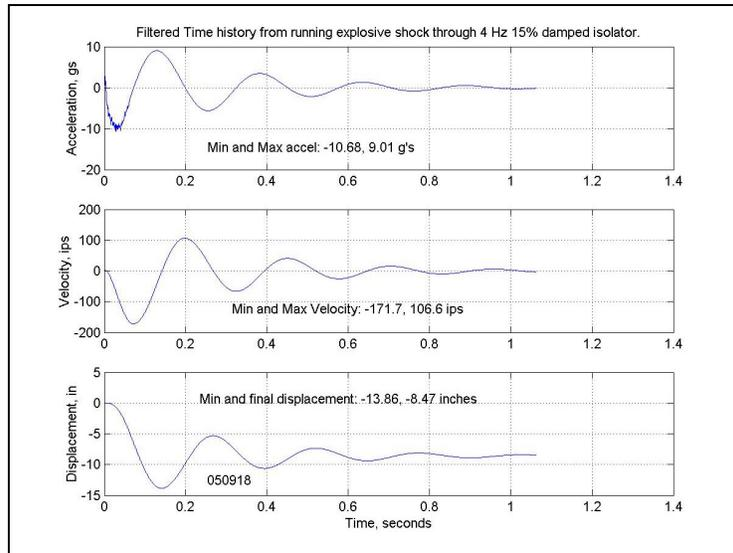
Figure 8a. The motion of a 4 Hz, 15% damped SDOF mass exposed to the shock of Figure 7b.
