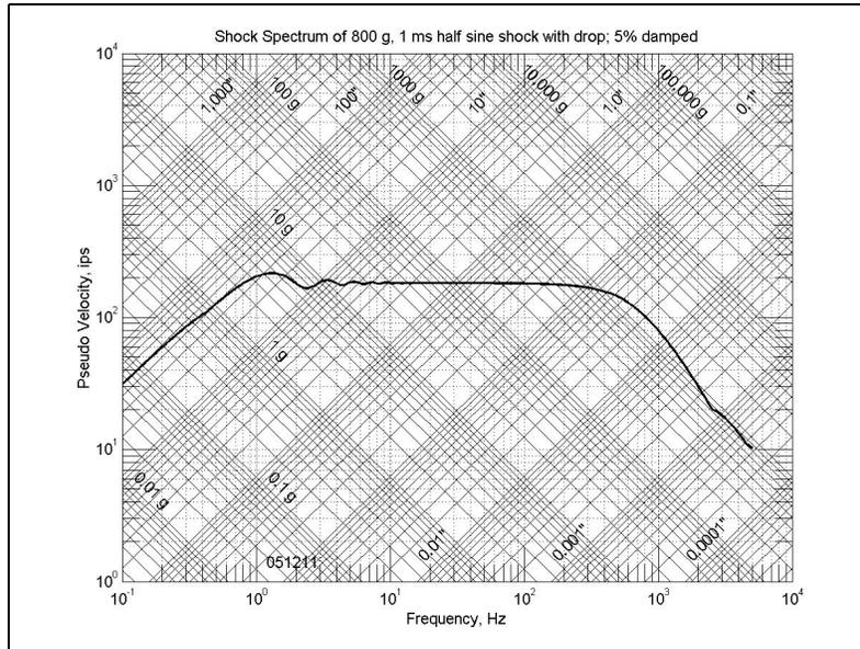
Figure 4. PVSS on 4CP for the half sine shock of Figure 3. Notice the high frequency asymptote is on the constant 800 g line, that the velocity plateau is at a little under 196 ips, and that the low frequency asymptote is on a constant displacement line of about 50 inches
