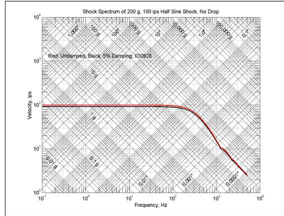
Figure 13b. The PVSS of a 200g, 100 ips half sine acceleration shock. In the lower right corner the spectra are asymptotic to 200g’s. From a little under 200 Hz down to 0.1 Hz the spectra show a constant velocity of 100 ips. That probably can not be.
