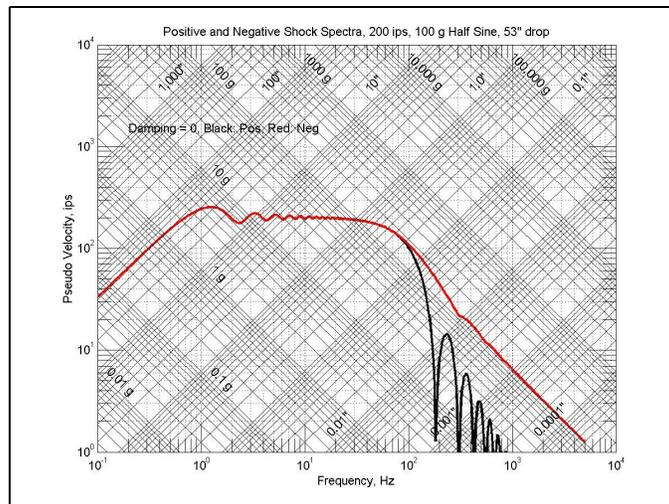
Figure 5a. Positive and negative PVSS for an undamped 200 ips, 100g, half sine. The negative spectrum only exceeds the positive at high frequencies where the PV is low.
