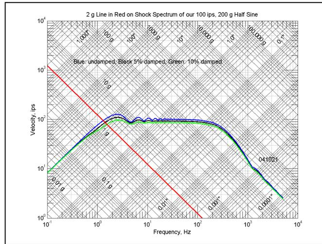
Figure 14b. Shock spectrum of a 100 ips, 200g half sine with the correct drop included.
