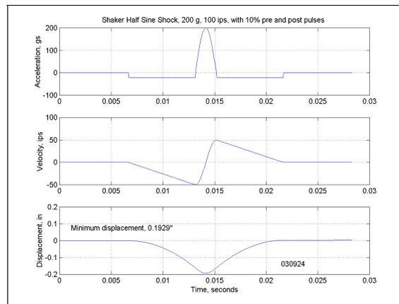
Figure 16a. Acceleration time history with 10% rectangular pre and post pulses to accomplish the 200g, 100 ips half sine shock on a shaker.
