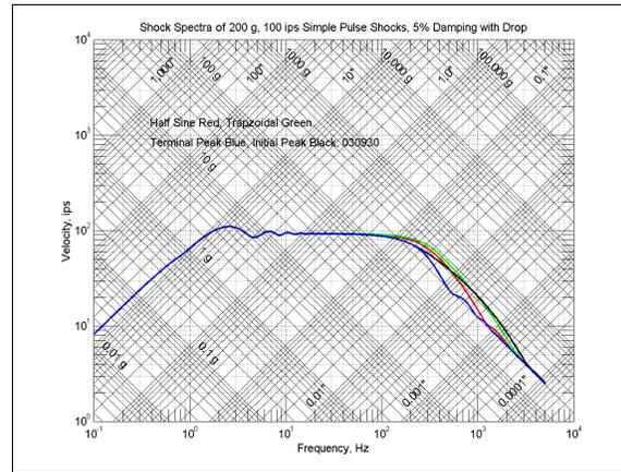
Figure 15b. Composite 5% damped shock spectrum plots of the half sine, the trapezoid, the initial peak and the terminal peak saw tooth shocks.
