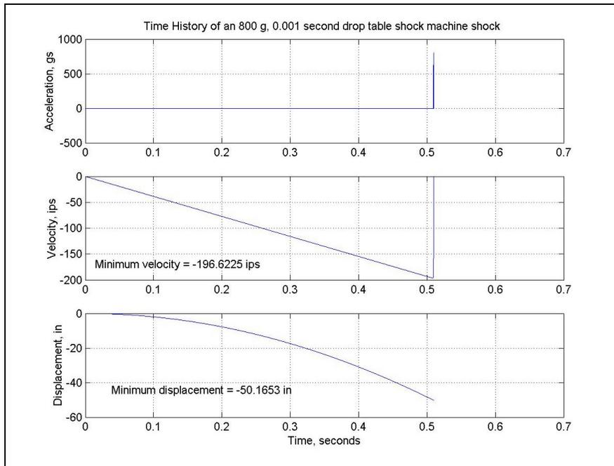
Figure 3. Time history of acceleration, velocity, and displacement of a drop table shock machine half sine shock.
