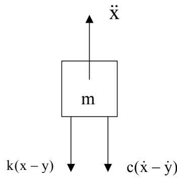
The free body diagram of the mass is in Fig. 2.
