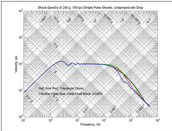
Figure 15a. Composite undamped shock spectrum plots of the half sine, the trapezoid, the initial peak and the terminal peak saw tooth shocks.
