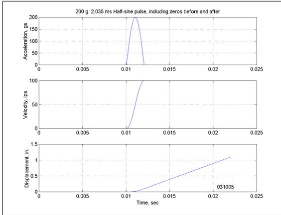
Figure 13a. Acceleration, velocity, and displacement of a half sine acceleration shock preceded and followed by zeros. The shock has a peak “g” level of 200g’s, and a velocity change of 100 ips; and continues at this velocity forever.
