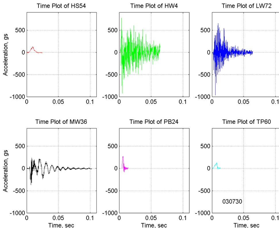
Figure 11. Here are the time histories of all six shocks. All but LW72 failed the blower. This should cure you from trying to estimate the severity of a shock in term of its g's.
