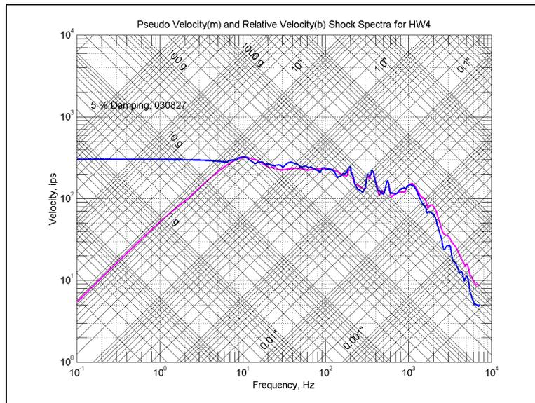
Figure 6. This is a superposition of the PVSS and the relative velocity shock spectrum for a 5% damped explosive shock.
